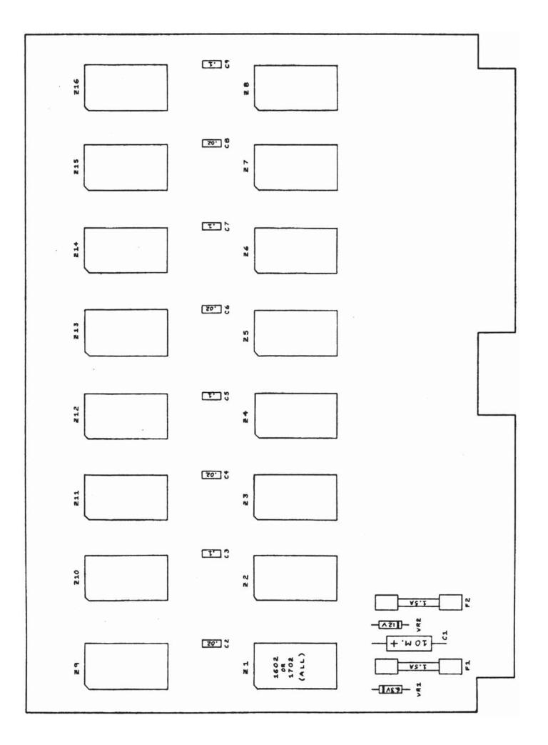
ignated as Zl through Zl6. Each ROM/PROM position corresponds to a "page" in memory - with Al being the position for the lowest "page" address on the card and Zl6 being the position for the highest page address on the card. When a ROM/PROM is to be installed, select the correct position on the card for the "page" address in memory for which the program on the prom is designed to operate. Install a 24 pin integrated circuit socket on the card and solder the socket pins. Then install the ROM/PROM.
