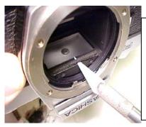
On this Yashica, you can see how I use an X-Acto knife to remove old damper material. I have seen people try to place paper and other items in this area to try to protect the focus screen, but I do not suggest doing this. It is too easy to trap a bit of old foam underneath a piece of paper and smear it on your focus screen. A false sense of security can become a liability quickly. Just work carefully and slowly.
